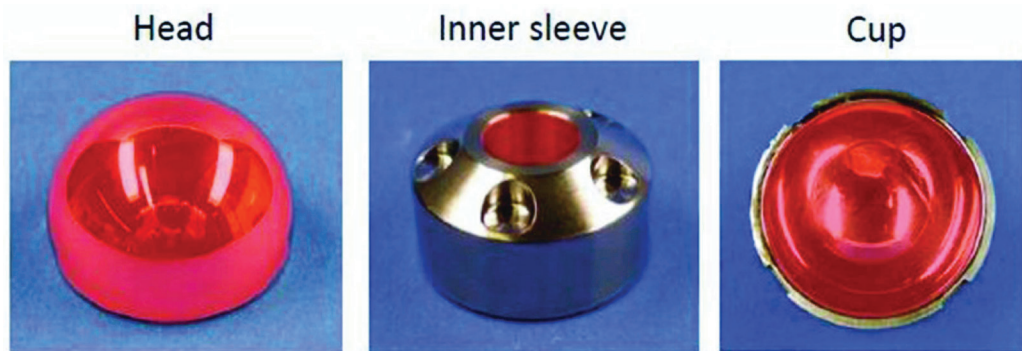
Figure 1. The red marked bearing and taper surfaces in the picture below were analyzed
