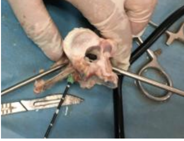
Figure 2 Set-up for the temperature measurement at zone 4 and the posterior wall. Left to right: zone 4 temperature probe, ablation needle, posterior wall temperature probe. The hole for the probe for the posterior wall is drilled through the lamina vertebralis.
