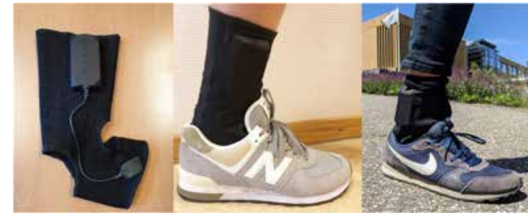
Figure 1: Overview of the IMUs embedded in socks. The sensor system consisted of a large casing (positioned above the lateral malleolus) containing the battery and memory drive, which was connected to the IMU on the dorsum of the foot via a small cable (left panel).
