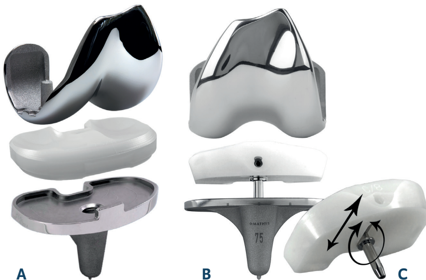
Figure 1. balanSys CR Knee system with a a fixed bearing, and b, c a mobile bearing (anterior-posterior (AP)-gliding (7-9 mm) and rotational (15°) degrees of freedom)
